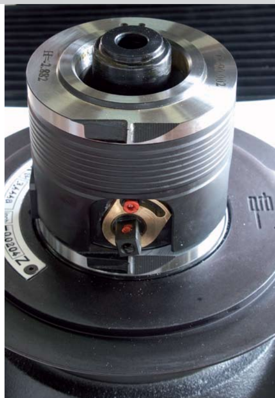
Original design HSK reduction sleeves with mechanical clamping system.
