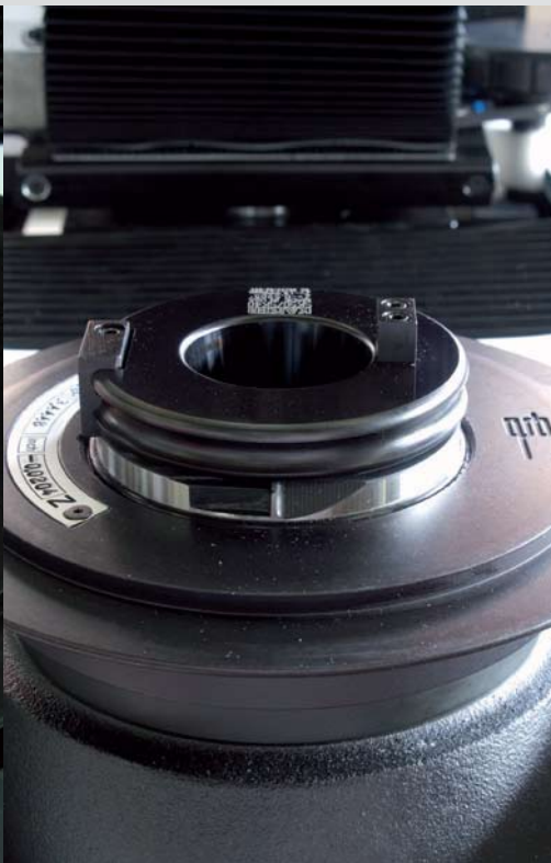
Range of reduction sleeves for ISO to ISO, ISO to VDI, ISO to KM, etc.
